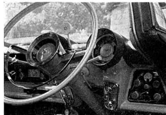
This tailor-made mobile installation was designed and constructed by G3HRO, and has won a number of awards at mobile rallies and at the 1961 Radio Hobbies Exhibition. The receiver to the left of the picture is fully transistorized, and covers the broadcast and six amateur bands. The six band transmitter runs 60 watts input to the p.a. with only four valves and a 30 watt transistor modulator. A full description of this equipment has appeared in Wireless World . (Photo by G3HRO)
